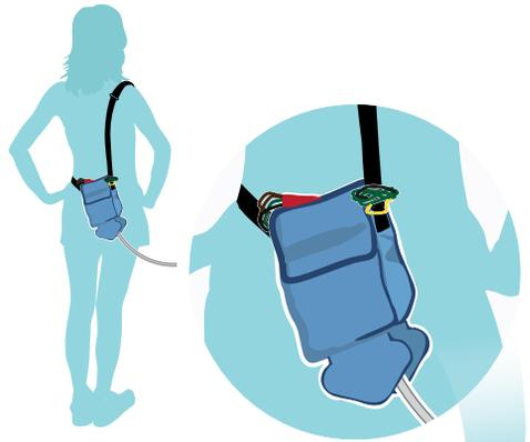
The box sends brain wave information to a receiver. The box and the receiver are connected with a cord. This cord must always be plugged in to the receiver so that we do not miss any information.
